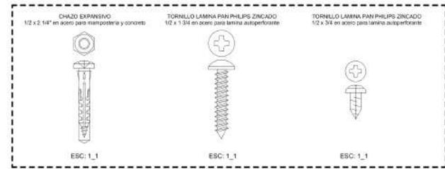
DMC 04 DETALLE ANCLAJE A MURO
