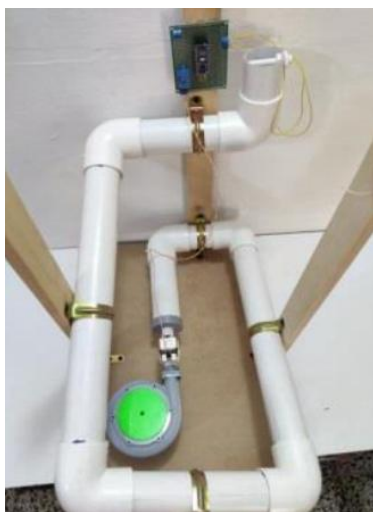
Figura 1. Drainage System for Power Generation
